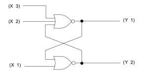
Figure 1-5 NOR Flip-Flop with Reset
